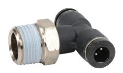
NITRA pneumatic push-to-connect fitting, branch tee, rotating, thermoplastic (PBT) body, nickel-plated brass threads, thread sealant, (1) 3/8in male NPT to (2) 1/4in push-to-connect. Package of 5.
