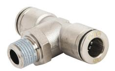
NITRA pneumatic push-to-connect fitting, branch tee, rotating, nickel-plated brass body, nickel-plated brass threads, thread sealant, (1) R1/8 male BSPT to (2) 1/4in push-to-connect. Package of 5.
