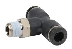
NITRA pneumatic push-to-connect fitting, branch tee, rotating, thermoplastic (PBT) body, nickel-plated brass threads, thread sealant, (1) 1/8in male NPT to (2) 1/4in push-to-connect. Package of 5.
