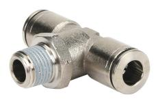
NITRA pneumatic push-to-connect fitting, branch tee, rotating, nickel-plated brass body, nickel-plated brass threads, thread sealant, (1) 1/8in male NPT to (2) 1/4in push-to-connect. Package of 5.
