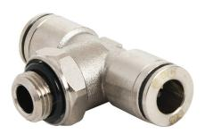
NITRA pneumatic push-to-connect fitting, male, branch tee, rotating, nickel-plated brass body, nickel-plated brass threads, thread sealant, (2) 1/4in push-to-connect to G1/8 BSPP. Package of 5.
