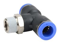
NITRA pneumatic push-to-connect fitting, branch tee, rotating, thermoplastic (PBT) body, nickel-plated brass threads, thread sealant, (1) R3/8 male BSPT to (2) 12mm push-to-connect. Package of 5.
