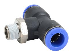
NITRA pneumatic push-to-connect fitting, branch tee, rotating, thermoplastic (PBT) body, nickel-plated brass threads, thread sealant, (1) R1/4 male BSPT to (2) 12mm push-to-connect. Package of 5.
