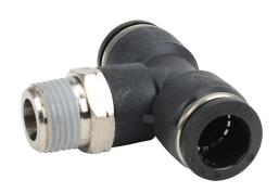
NITRA pneumatic push-to-connect fitting, branch tee, rotating, thermoplastic (PBT) body, nickel-plated brass threads, thread sealant, (1) 3/8in male NPT to (2) 1/2in push-to-connect. Package of 5.
