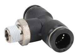
NITRA pneumatic push-to-connect fitting, branch tee, rotating, thermoplastic (PBT) body, nickel-plated brass threads, thread sealant, (1) 1/4in male NPT to (2) 1/2in push-to-connect. Package of 5.
