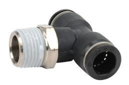
NITRA pneumatic push-to-connect fitting, branch tee, rotating, thermoplastic (PBT) body, nickel-plated brass threads, thread sealant, (1) 1/2in male NPT to (2) 1/2in push-to-connect. Package of 5.
