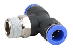
NITRA pneumatic push-to-connect fitting, branch tee, rotating, thermoplastic (PBT) body, nickel-plated brass threads, thread sealant, (1) R3/8 male BSPT to (2) 10mm push-to-connect. Package of 5.
