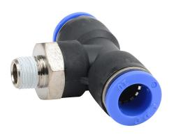
NITRA pneumatic push-to-connect fitting, branch tee, rotating, thermoplastic (PBT) body, nickel-plated brass threads, thread sealant, (1) R1/8 male BSPT to (2) 10mm push-to-connect. Package of 5.
