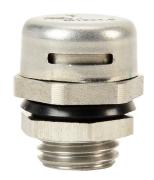
Bimed pressure relief vent plug, M12 x 1.5mm thread type, stainless steel, 417 mL/min @ 70 mBar (1 psi), IP67 IP68, UL Type 4X, 12 and 13.
