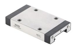
WON MB7 series wide mini bearing block, full ball recirculating, rectangular long, end seal, stainless steel. For use with MB7 series rails.
