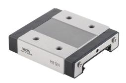
WON MB12 series wide mini bearing block, full ball recirculating bearing, rectangular, end seal, stainless steel. For use with MB12 series rails.
