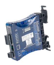
AutomationDirect Modbus gateway, Ethernet to serial, (1) Ethernet 10/100Base-T (RJ45) and (1) RS-422/485 (6-pin terminal) port(s), (12) simultaneous Ethernet connections, (128) serial device(s), 12-24 VDC required.
