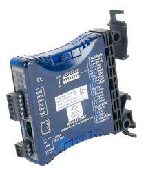
AutomationDirect Modbus gateway, Ethernet to serial, (1) Ethernet 10/100Base-T (RJ45) and (1) RS-422/485 (6-pin terminal) port(s), (12) simultaneous Ethernet connections, (128) serial device(s), 12-24 VDC required.
