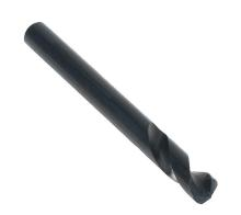
MK Morse pilot drill bit, replacement, 1/4in, split point, high-speed steel (HSS), black oxide finish, round shank, 3-3/32in overall length. For use with all MK Morse arbors.
