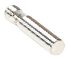
ProSense magnetic proximity sensor, tubular, 12mm diameter x 60mm body, stainless steel housing, PNP, N.O. output, 60mm sensing distance, flush, 5 kHz switching frequency, IP65 IP68 IP69K, 4-pin M12 quick-disconnect.
