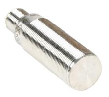
ProSense magnetic proximity sensor, tubular, 18mm diameter x 60mm body, stainless steel housing, PNP, N.O. output, 70mm sensing distance, flush, 5 kHz switching frequency, IP65 IP68 IP69K, 4-pin M12 quick-disconnect.
