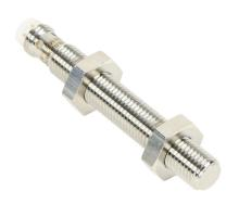
ProSense magnetic proximity sensor, tubular, 8mm diameter x 60mm body, 316L stainless steel housing, PNP, N.O. output, 60mm sensing distance, flush, 5 kHz switching frequency, IP67, 3-pin M8 quick-disconnect.
