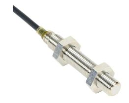
ProSense magnetic proximity sensor, tubular, 8mm diameter x 50mm body, 316L stainless steel housing, PNP, N.O. output, 60mm sensing distance, flush, 5 kHz switching frequency, IP67, pigtail.
