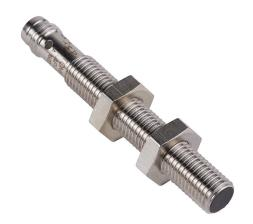
AutomationDirect magnetic proximity sensor, tubular, 8mm diameter x 60mm body, 316L stainless steel housing, PNP, N.O. output, 60mm sensing distance, flush, 5 kHz switching frequency, IP67, 3-pin M8 quick-disconnect.
