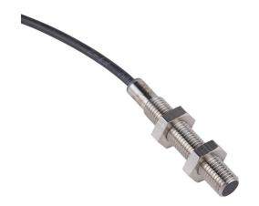
AutomationDirect magnetic proximity sensor, tubular, 8mm diameter x 50mm body, 316L stainless steel housing, PNP, N.O. output, 60mm sensing distance, flush, 5 kHz switching frequency, IP67, pigtail.
