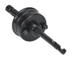
MK Morse arbor assembly, 5/8-18 UNF, 3/8in hex shank. For use with 1-1/4in and above hole saws. Spring loaded pin drive arbor and 1/4in high-speed steel (HSS) pilot bit included.
