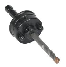
MK Morse arbor assembly, 5/8-18 UNF, 3/8in hex shank. For use with 1-1/4in and above hole saws. Spring loaded pin drive arbor and 1/4in carbide-tipped pilot bit included.
