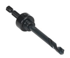
MK Morse arbor assembly, 1/2-20 UNF, 1/4in hex shank. For use with 9/16in to 1-13/16in hole saws. Standard arbor and 1/4in high-speed steel (HSS) pilot bit included.
