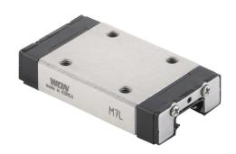
WON M7 series mini bearing block, full ball recirculating, rectangular long, end seal, stainless steel. For use with M7 series rails.
