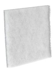
Fandis filter, replacement,  $8.43 \times 8.43$ in, synthetic fiber, washable, G4 (coarse). Package of 6. For use with Fandis FF15 filter fans and exhaust grilles.
