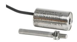
Alliance Sensors inductive linear position sensor, fixed slide, 6.4mm stroke, 5.2mm shaft diameter, 4-20 mA output, 19mm diameter x 35mm body, M5 x 0.8 mount, pigtail, 3.2ft/1m cable length.
