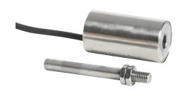
Alliance Sensors inductive linear position sensor, fixed slide, 2.5mm stroke, 5.2mm shaft diameter, 4-20 mA output, 19mm diameter x 35mm body, M5 x 0.8 mount, pigtail, 3.2ft/1m cable length.
