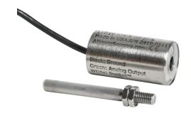
Alliance Sensors inductive linear position sensor, fixed slide, 25mm stroke, 5.2mm shaft diameter, 4-20 mA output, 19mm diameter x 35mm body, M5 x 0.8 mount, pigtail, 3.2ft/1m cable length.
