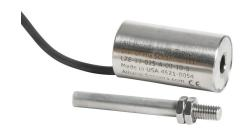
Alliance Sensors inductive linear position sensor, fixed slide, 25mm stroke, 5.2mm shaft diameter, 0-10 VDC output, 19mm diameter x 35mm body, M5 x 0.8 mount, pigtail, 3.2ft/1m cable length.
