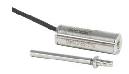
Alliance Sensors inductive linear position sensor, fixed slide, 25mm stroke, 4mm shaft diameter, 0-10 VDC output, 12.7mm diameter x 35.8mm body, M4 x 0.7 mount, pigtail, 3.2ft/1m cable length.
