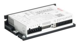
Ever Motion Solutions DC open loop advanced microstepping stepper drive, 10A per phase, 2-phase output, 24-80 VDC, bipolar, position mode, 200 to 51200 steps per revolution.
