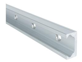
SureMotion LUV-2 series guide track, anodized aluminum, 19.74 x 40 x 1520mm. For use with SureMotion LUV-2 series v-carriages.
