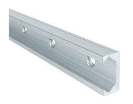
SureMotion LUV-2 series guide track, anodized aluminum, 19.74 x 40 x 1120mm. For use with SureMotion LUV-2 series v-carriages.
