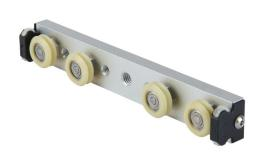
SureMotion LUV series v-carriage, single row ball bearing, 4-wheel, end seal, polyacetal/440C stainless steel. For use with SureMotion LUV-1 series guide tracks.
