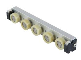
SureMotion LUC series crown carriage, single row ball bearing, 5-wheel, end seal, polyacetal/440C stainless steel. For use with SureMotion LUC-0 series guide tracks.
