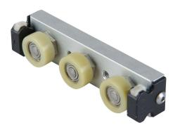
SureMotion LUC series crown carriage, single row ball bearing, 3-wheel, end seal, polyacetal/440C stainless steel. For use with SureMotion LUC-0 series guide tracks.
