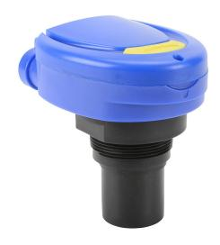
Flowline EchoSpan ultrasonic liquid level sensor, 32.8ft/10m sensing range, 4-20 mA, 12-28 VDC operating voltage, LCD digital display with pushbuttons, 2in male NPT process connection.
