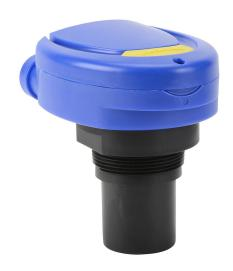
Flowline EchoSpan ultrasonic liquid level sensor, 26.2ft/8m sensing range, 4-20 mA, 12-28 VDC operating voltage, LCD digital display with pushbuttons, 2in male NPT process connection.
