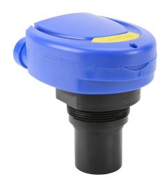
Flowline EchoSpan ultrasonic liquid level sensor, 18ft/5.5m sensing range, 4-20 mA, 12-28 VDC operating voltage, LCD digital display with pushbuttons, 2in male NPT process connection.
