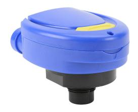
Flowline EchoSpan ultrasonic liquid level sensor, 9.8ft/3m sensing range, 4-20 mA, 12-28 VDC operating voltage, LCD digital display with pushbuttons, 1in male NPT process connection.
