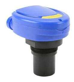
Flowline EchoSwitch ultrasonic liquid level sensor, 26.2ft/8m sensing range, 4-20 mA or (1) SPDT relay, (2) SPST-N.O. relays, 95-250 VAC operating voltage, LCD digital display with pushbuttons, 2in male NPT process connection.
