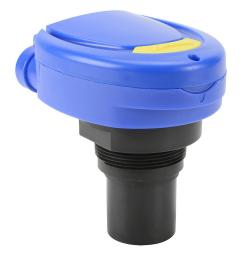
Flowline EchoSwitch ultrasonic liquid level sensor, 18ft/5.5m sensing range, 4-20 mA or (1) SPDT relay, (2) SPST-N.O. relays, 95-250 VAC operating voltage, LCD digital display with pushbuttons, 2in male NPT process connection.
