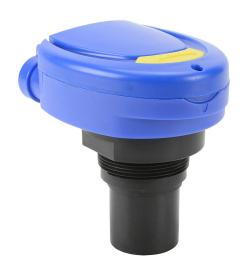
Flowline EchoSwitch ultrasonic liquid level sensor, 18ft (5.5m) sensing range, 4-20 mA or (1) SPDT relay, (2) SPST-N.O. relays, 95-250 VAC operating voltage, LCD digital display with pushbuttons, 2in male NPT process connection.
