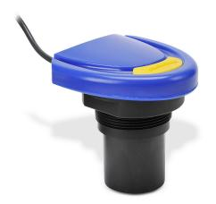
Flowline EchoSonic II ultrasonic liquid level sensor, 32.8ft/10m sensing range, 4-20 mA, 14-28 VDC operating voltage, 2in male NPT process connection.
