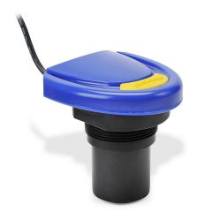
Flowline EchoSonic II ultrasonic liquid level sensor, 26.2ft/8m sensing range, 4-20 mA, 14-28 VDC operating voltage, 2in male NPT process connection.
