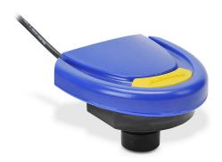
Flowline EchoSonic II ultrasonic liquid level sensor, 9.8ft (3m) sensing range, 4-20 mA, 14-28 VDC operating voltage, 1in male NPT process connection.
