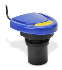
Flowline EchoSonic II ultrasonic liquid level sensor, 18ft/5.5m sensing range, 4-20 mA, 14-28 VDC operating voltage, 2in male NPT process connection.
