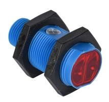
Contrinex photoelectric sensor, tubular, threaded, diffuse, visible red light emission, 3-1200mm sensing distance, complementary light-on/dark-on, PNP, potentiometer, 1.5 kHz switching frequency, ABS plastic housing, 4-pin M12 quick-disconnect.
