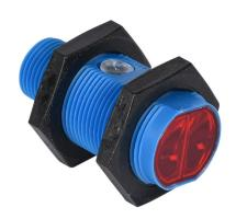
Contrinex photoelectric sensor, tubular, threaded, diffuse, visible red, 3-1200mm sensing distance, complementary light-on/dark-on, PNP, potentiometer, 1.5 kHz switching frequency, ABS plastic housing, 4-pin M12 quick-disconnect.
